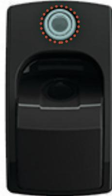
Once scan is finished remove finger and wait for the 'halo' button to change colour.
