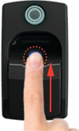
Place finger on sensor to activate (the sensor will illuminate).
